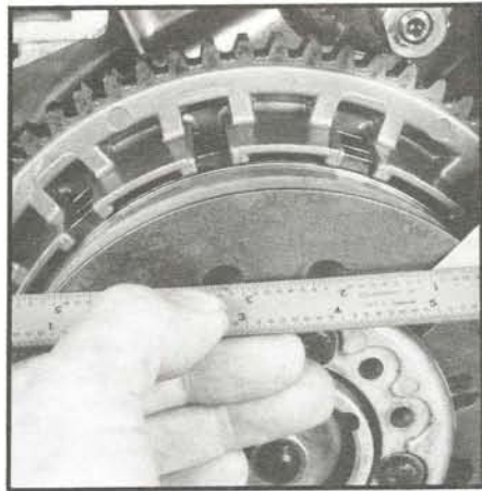
Clutch spring shape can be measured with ordinary tools. Note that the four spring retaining bolts are fitted through holes with a letter—either A, B, or C. These hole sets pre-load the spring different amounts, changing its shape. Best lever feel results when the spring is flat or slightly dished (left photo). The large contact area of the new clutch hub eliminates wear and the sticking between the plates and hub.
