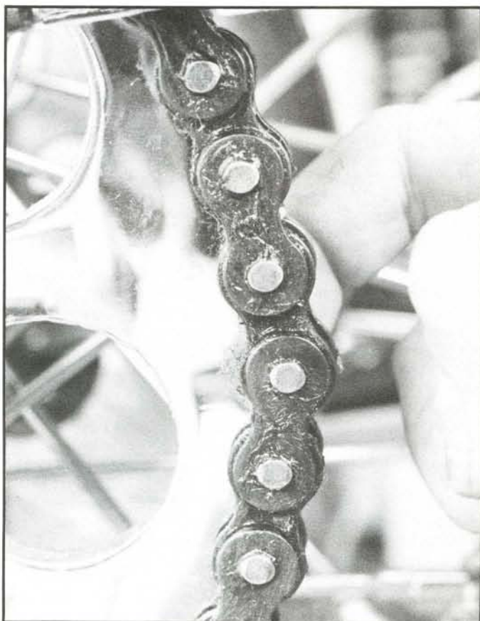
This sprocket was cut wrong an' it's gonna take the chain out in a few thousand miles. Sorry, bro, but there ain't very many good chain wheels bein' made these days, includin' the factory's — which this one is.
