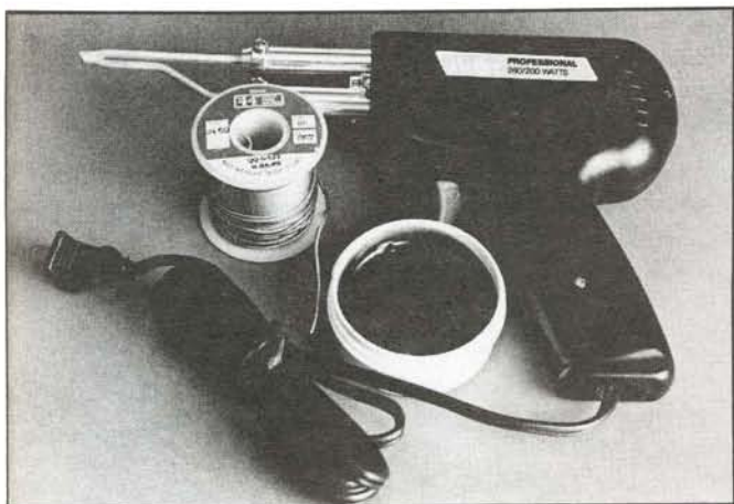
Get a good soldering gun, some resin-core solder, and a little non-acid flux—you're on your way.
