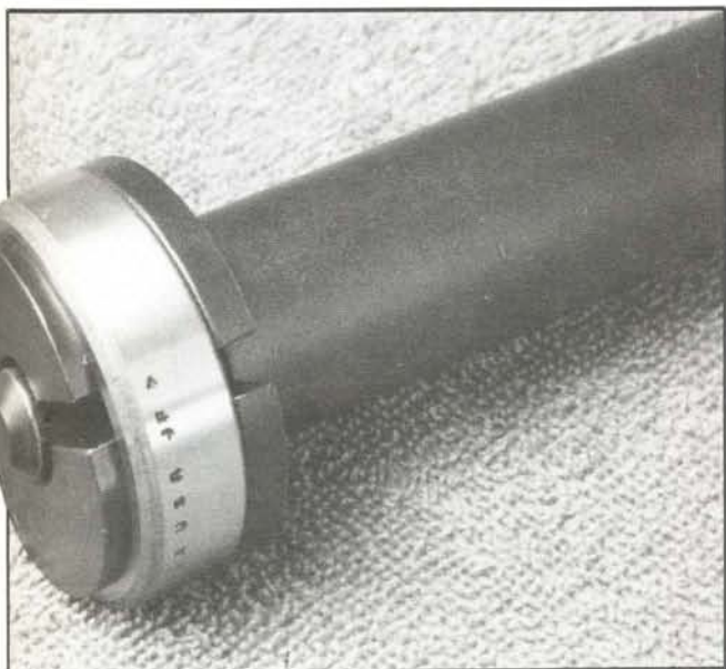
H-D makes this outer race driver. Nice tool — you oughta get one.
