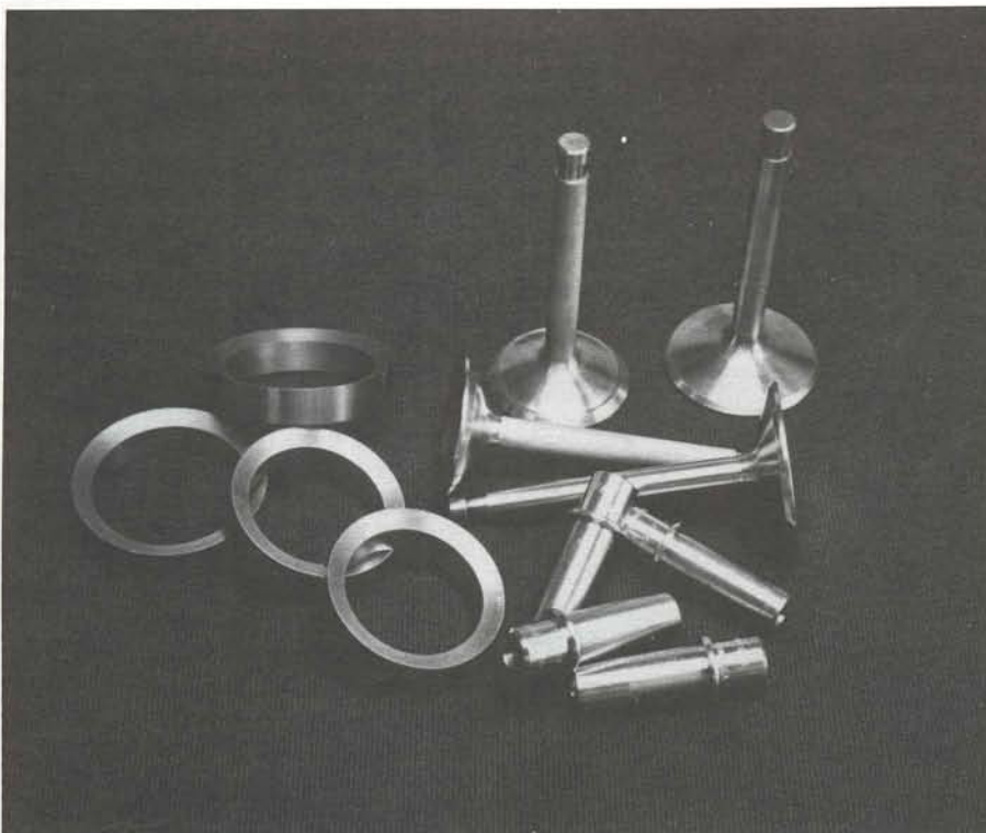
These valves, seats, and guides from Branch Flowmetrics are made of the best modern materials. They will more than double the life of a shovelhead valve job.
