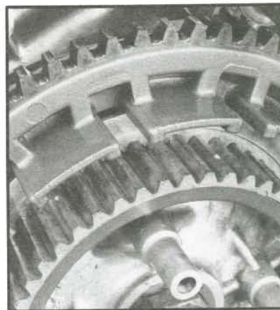
Clutch spring shape can be measured with ordinary tools. Note that the four spring retaining bolts are fitted through holes with a letter—either A, B, or C. These hole sets pre-load the spring different amounts, changing its shape. Best lever feel results when the spring is flat or slightly dished (left photo). The large contact area of the new clutch hub eliminates wear and the sticking between the plates and hub.
