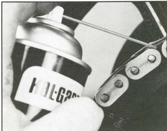
Squirtin' lube all over the outside of yer chain won't help much — it's gotta get inside. All them Harley power-pulses go through the pins and bushings inside the chain.
