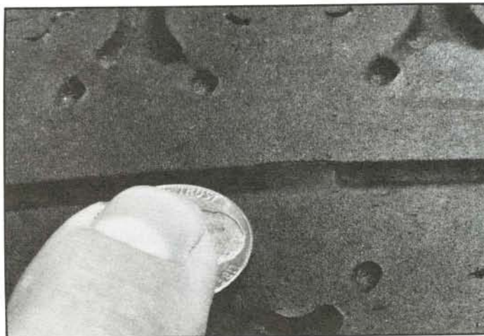
You'll need a new tire when the wear bar is flush with the tread surface or the tread depth is equal to the width of a new nickel. While ya might get away with runnin' a tire till it's bald, you are takin' a chance on eventually slidin' yer ass down the road.
