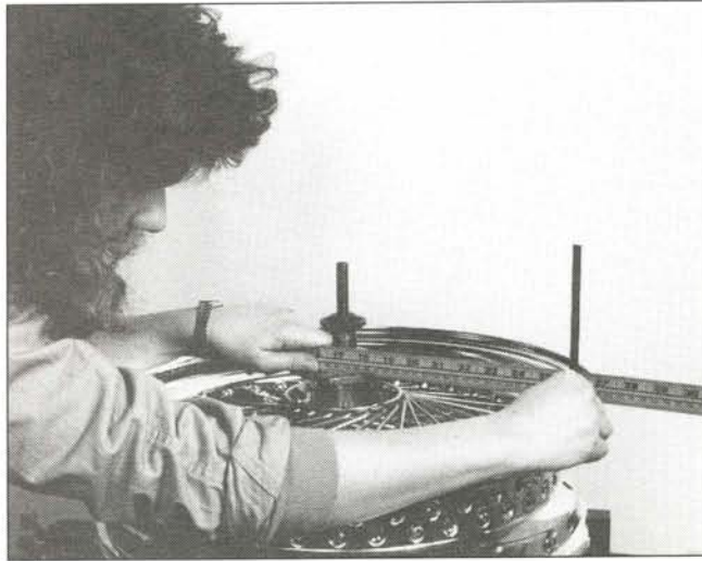
With all 80 spokes loose in the rim, Brook uses a straightedge to set the required offset of the hub to the rim.
