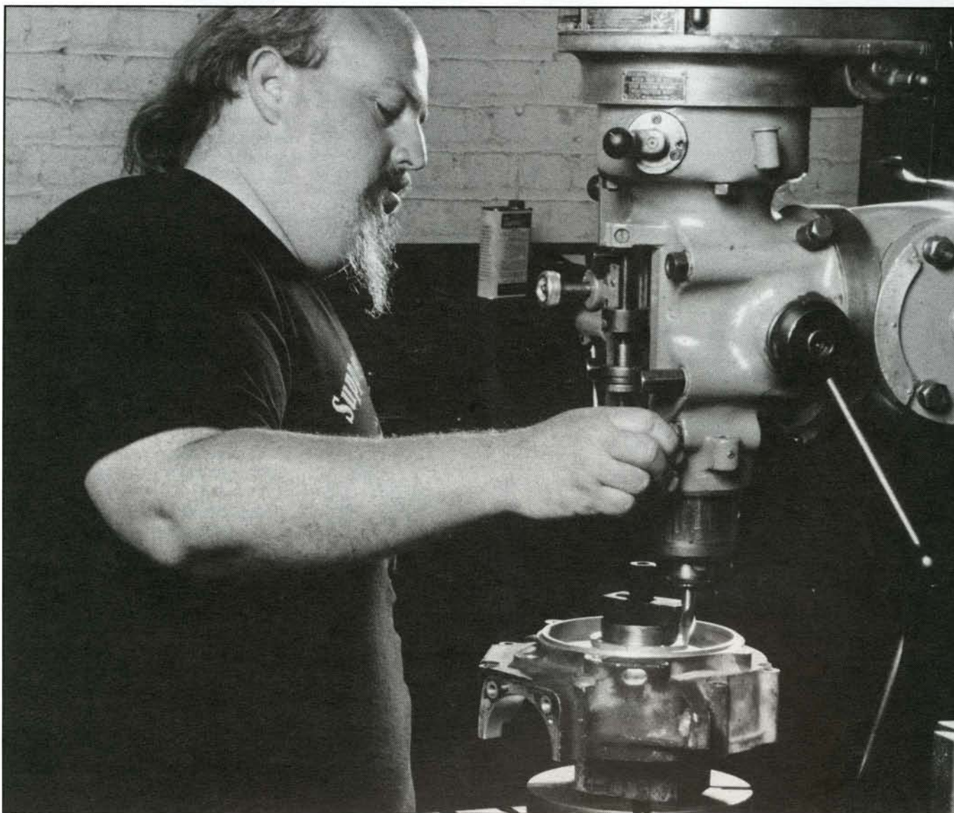
Giggie, the master mechanic at Departure Bike Works in Richmond, Virginia, (804) 231-0244, prepares to machine the case.
