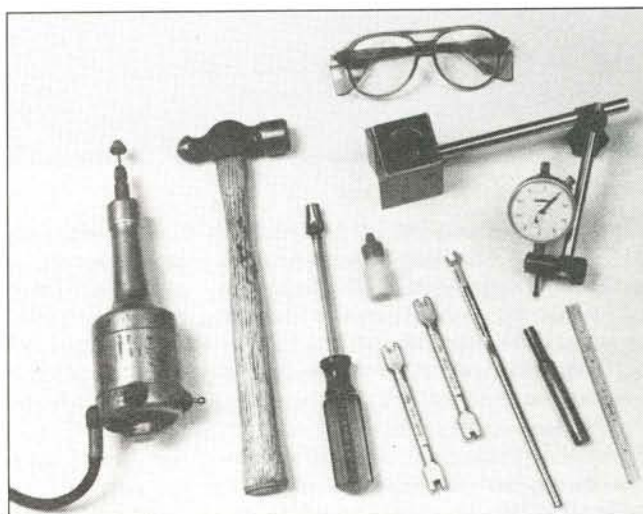
Hand tools needed to complete a wheel. Brook had to make her spoke wrench to work on an 80-spoke wheel.
