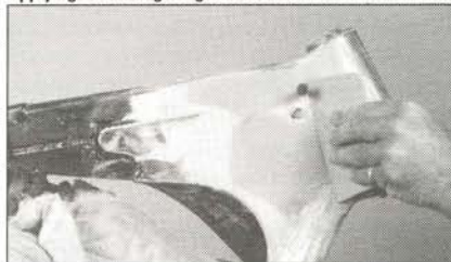
Bondo work complete and coats of primer being applied to allow inspection of work.
